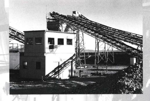
Personnel and equipment within the control rooms are isolated from high temperatures, dirt and noise. The building is self-contained, complete with emergency power systems, housing the computerized operating system at this automated cement batch plant.
